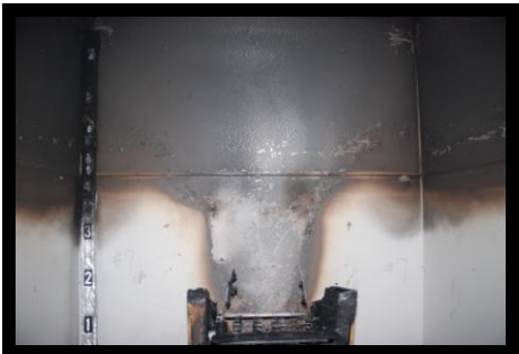
Figure 12: Chair 7 42" Header - Actual Damage (left); Calcination Measurements (center); Thermocouple Data (right)
