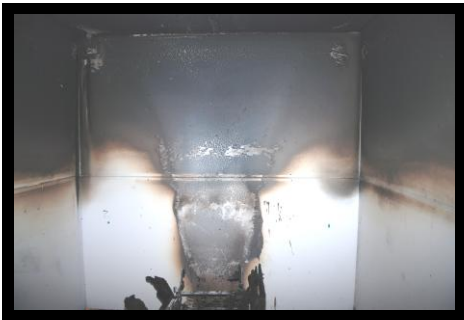
Figure 7: Chair 2 18" Header - Actual Damage (left); Calcination Measurements (center); Thermocouple Data (right)
