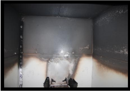
Figure 14: Chair 9 42" Header - Actual Damage (left); Calcination Measurements (center); Thermocouple Data (right)
