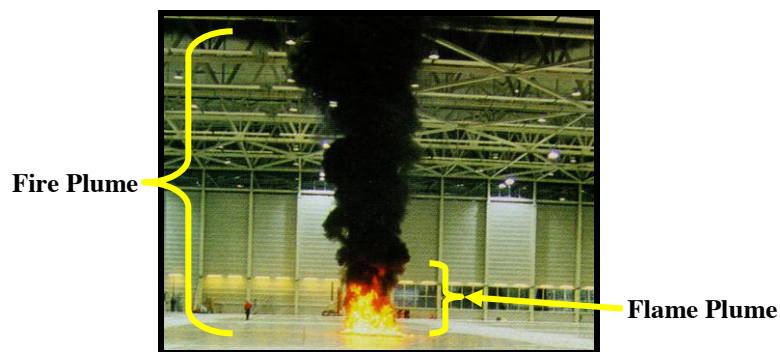
Figure 1: Flame Plume and Fire Plume
