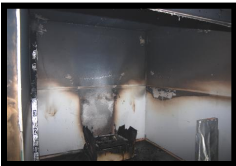
Figure 8: Chair 3 18" - Actual Damage (left); Calcination Measurements (center); Thermocouple Data (right)
