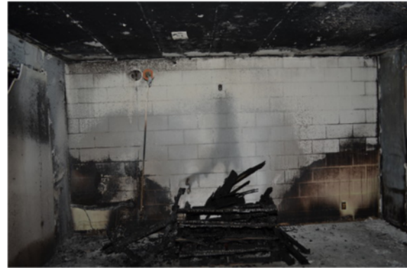
Fig. 6 Photograph of a Conical-Shaped Fire Pattern along a concrete block wall (fire origin was located under the stack of wooden pallets-fire test conducted at ECU by author)
