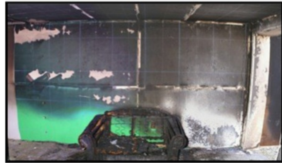
Fig. 13 Ventilation-Generated Fire Pattern near open doorway (fire origin located across room-fire test conducted at ECU by author)
