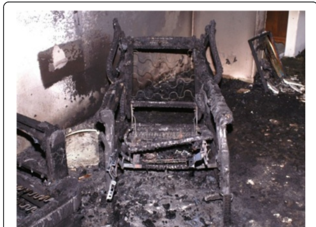
Fig. 14 Pre-fire Drywall Repairs Influencing the Post-fire Visible Damage to the Wall (fire origin located along front of chair-fire test conducted at ECU by author)
