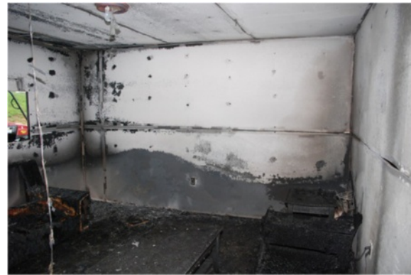
Fig. 12 Upper Layer-Generated Fire Pattern (fire origin was located along adjacent wall-fire test conducted at ECU by author)
